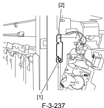
2) Remove the screw [1] and disconnect the connector [2].
