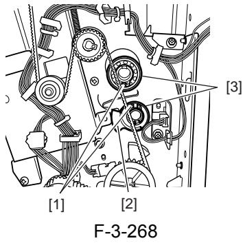
7) Remove the two C-rings [1] at the front and remove the two gears [2].
