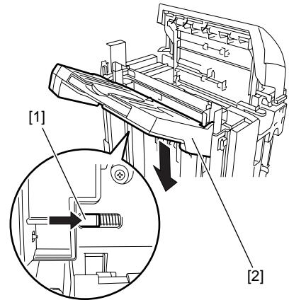
**⚠** When installing the tray, be careful not to twist the tray cable. To prevent the gear phase from shifting due to the front and rear rails, the tray must be attached horizontally. Lower the tray [1] to the position shown in the figure and compare the heights of the shutter guide top edges [2] with those of the tray projections [3] at the front and rear to check that the tray is attached horizontally. If their heights are not the same, remove the tray and then attach it again.
