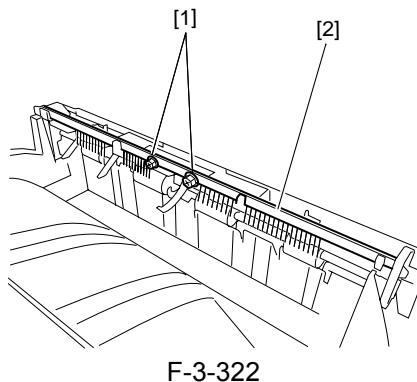
**⚠**A ground plate [1] is provided in the area where the escape delivery static charge eliminator [2] is mounted. When mounting the escape delivery static charge eliminator [2], insert it in the lateral direction.
