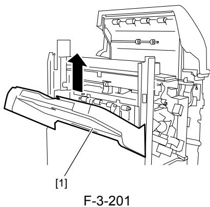
to push the tray lift motor gear [1] to the front (using a screwdriver or the like) to release the clutch. However, when the clutch is released, the tray [2] drops by its own weight. Be sure to hold the tray with your hand when releasing the clutch.
