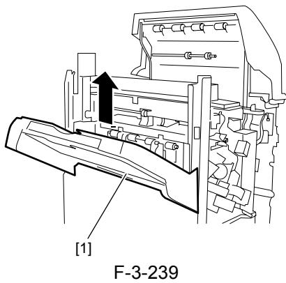
**⚠**When installing the tray, be careful not to twist the tray cable. To prevent the gear phase from shifting due to the front and rear rails, the tray must be attached horizontally. Lower the tray [1] to the position shown in the figure and compare the heights of the shutter guide top edges [2] with those of the tray projections [3] at the front and rear to check that the tray is attached horizontally. If their heights are not the same, remove the tray and then attach it again.
