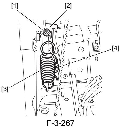
6) Remove the two C-rings [1] at the rear, and remove the sensor flag [2] and two bearings [3].
