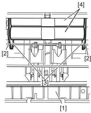
**⚠**When installing, attach the gear [2] so that the grooves [1] of the paper folding rollers face each other and align the phase.
