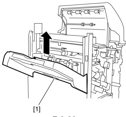
**⚠**When installing the tray, be careful not to twist the tray cable. To prevent the gear phase from shifting due to the front and rear rails, the tray must be attached horizontally. Lower the tray [1] to the position shown in the figure and compare the heights of the shutter guide top edges [2] with those of the tray projections [3] at the front and rear to check that the tray is attached horizontally. If their heights are not the same, remove the tray and then attach it again.
