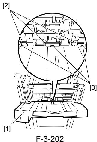
1) Remove screw [1] and remove the stopper [2].
