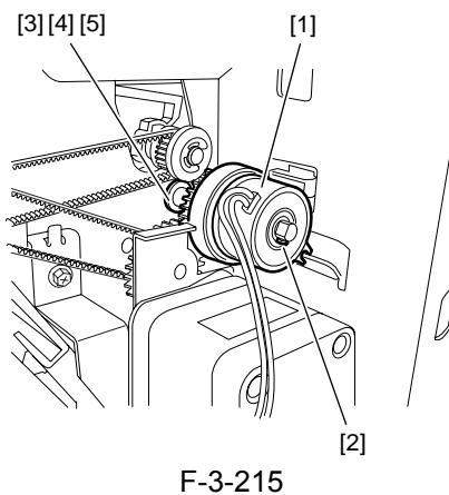
7) Disconnect two connectors [1] and remove harness from the clamp and edge saddle [2].
